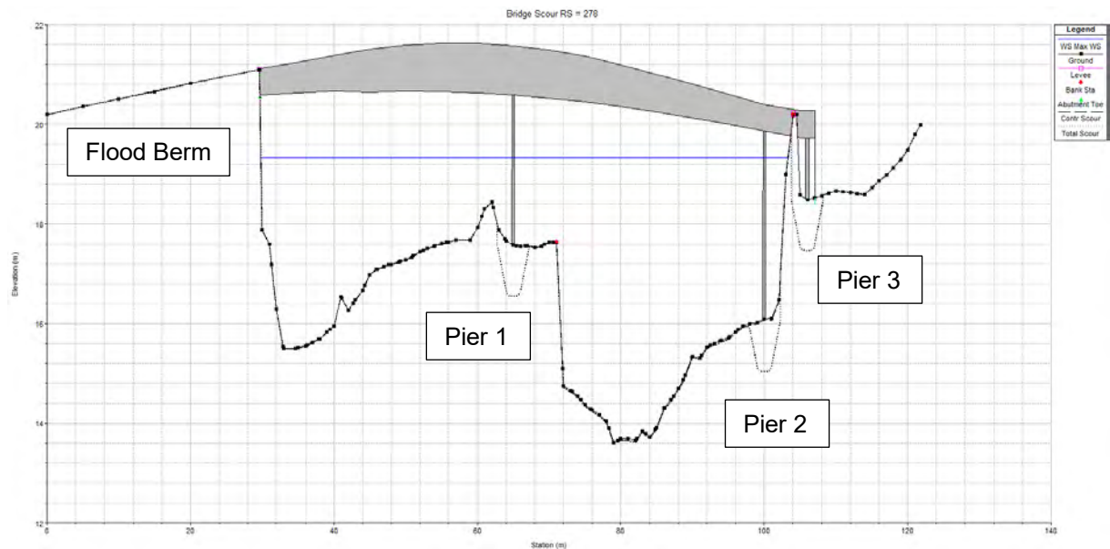
Figure 8-4: South Bridge scour depth (1% AEP, 0° Angle)
