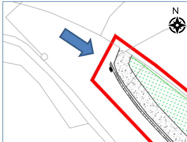
Figure 2-3 Extract Drawing 11007-2014-D01, showing end of wall and intersection with new pedestrian access point to the park
