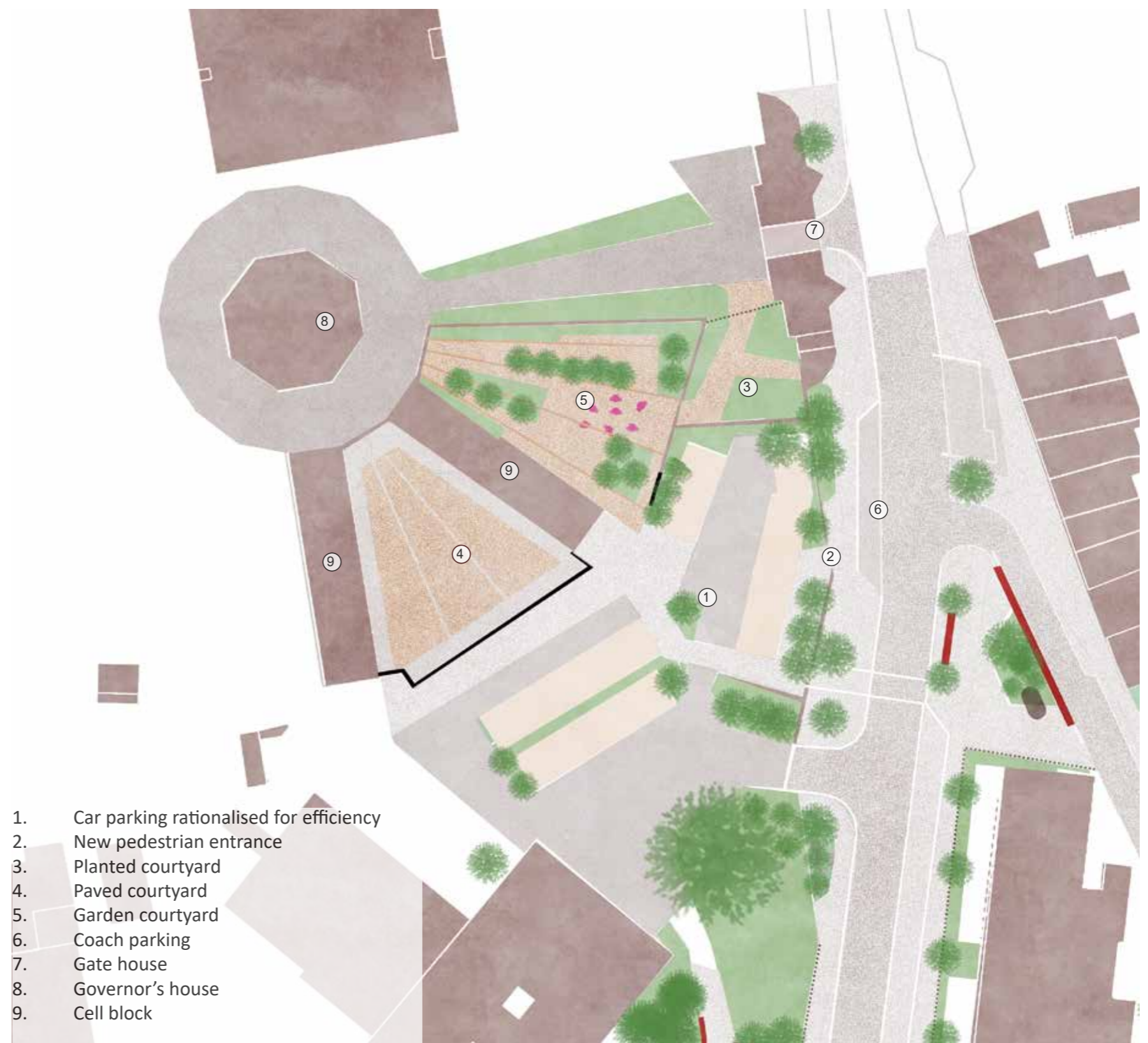
Landscape concept schematic Refer to Part 8 scaled drawings for details
