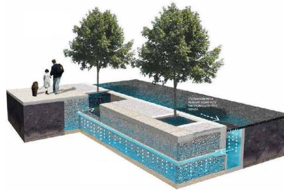
Structural tree pit diagram
